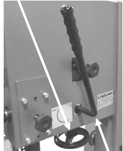
Quick action blade tension lever (activated)
